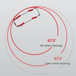
\* RTX with 173" wheelbase (wall-to-wall)
