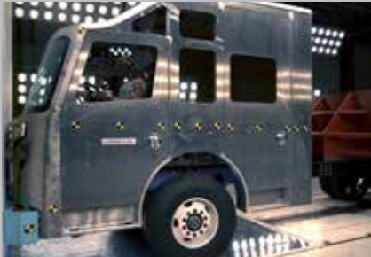
Frontal Impact Test
