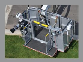
Ice and wind monitoring are standard. The T-Rex<sup>™</sup> is able to operate in wind speeds up to 39 MPH. The on-board CAN-bus electronic control system continuously measures the live load on the aerial and will automatically compensate for any ice build-up on the aerial device.
