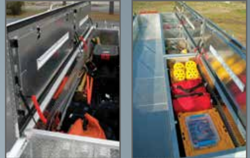
Roof compartments configured for mission specific equipment and equipped with recessed LED light and hold-open pneumatic spring on the lids.
