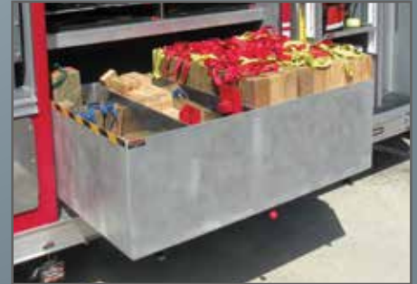
40" deep slide-out drawers in the bottom of the compartments are only available with a drop/pinch frame body or trailer.
