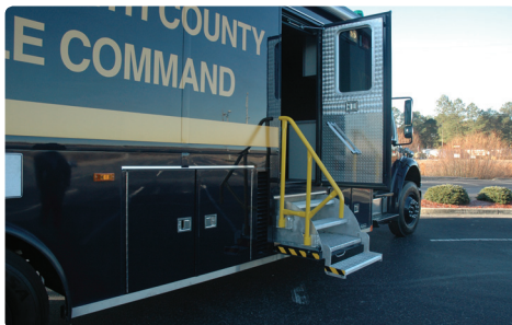
Drop-down entrance step provides OSHA compliant entrance and exiting of the interior without a cumbersome setup.
